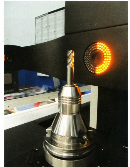
Somta Tools have purchased a Walter Helicheck Basic 3, a 4-axis CNC measuring machine for non-contact complete measurement of rotationally symmetrical precision tools with complex geometry
