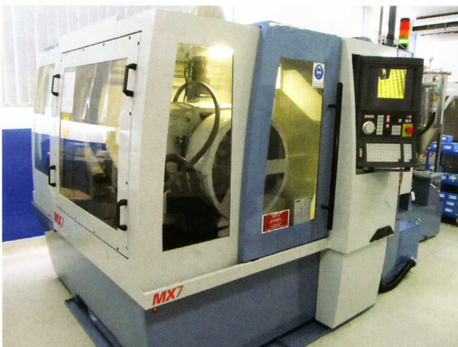
With the increased demand for product Somta Tools have now acquired an ANCA MX7 equipped with a 20kW motor and a robotic arm, to further increase production capacity and improve delivery times
