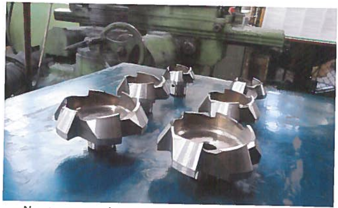
New purpose-made cutters from Somta Tools that were used in the extraction of the infected tusk
