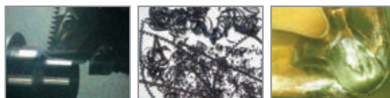
Conventional chip breaker
